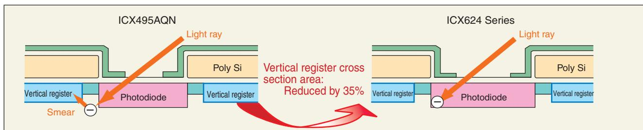
■ Figure 2 Vertical Register Structure Schematic Diagram
